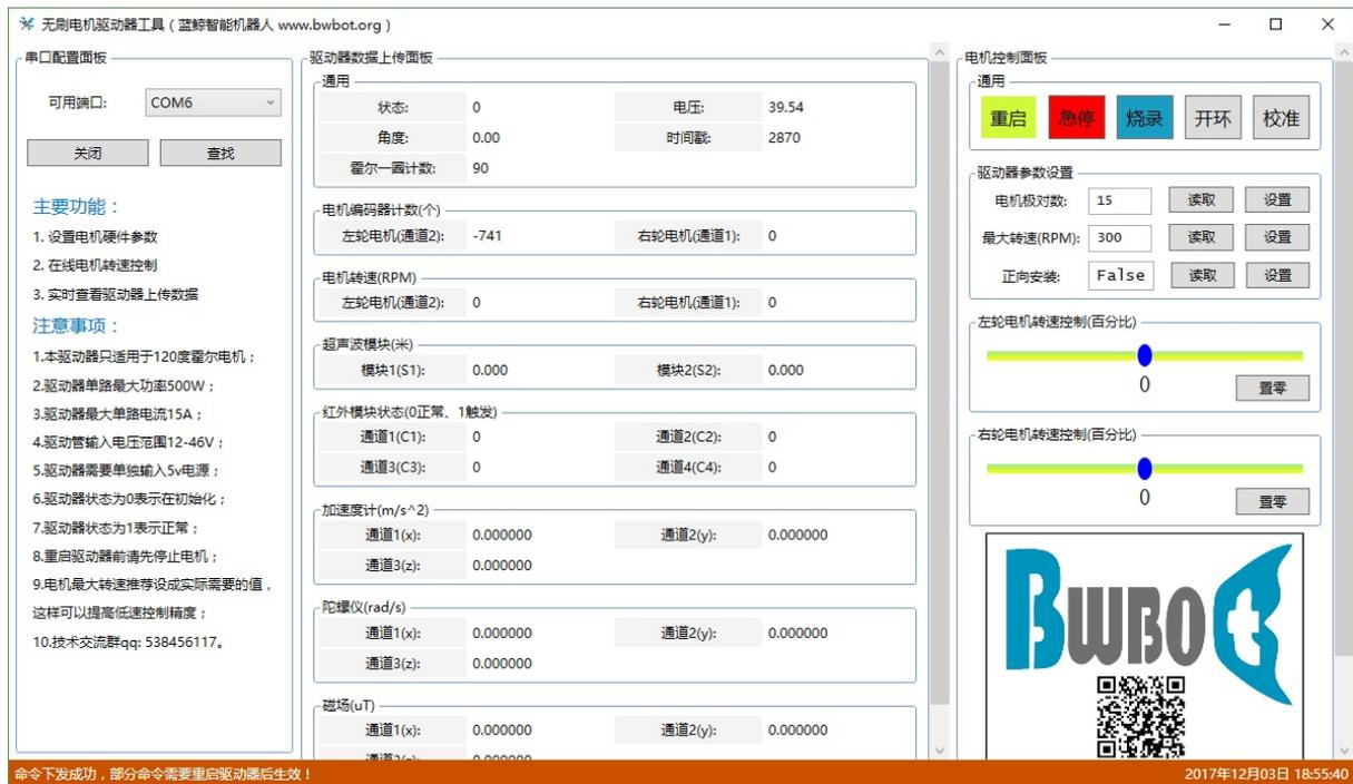
After the driver is powered on, there will be a period of initialization time, and the status will be 0. After the initialization is completed, the status will become 1, and the background color will become green. Only in this case can the "Control Panel" be operated.
