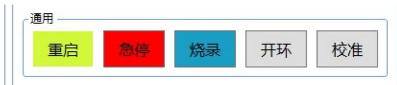
Click "open loop", the drive will temporarily enter the "speed open loop" control mode, at this time, the motor PWM switch value is directly proportional to the speed command. Restarting the drive will cause the drive to exit the "speed open loop" control mode and enter the default speed closed loop mode.
