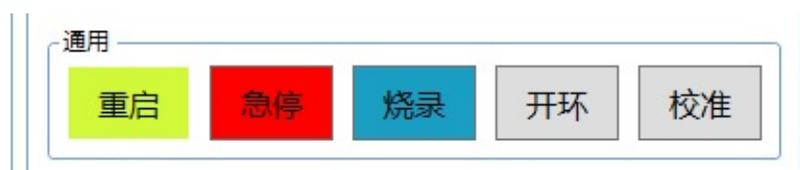
"Restart" makes the drive control chip restart, "e-stop" can brake two motors at the same time, "flash" configures the drive to be in the firmware update state, "open loop" temporarily configures the drive to speed open-loop control mode, and "calibration" starts the drive IMU automatic calibration program.
