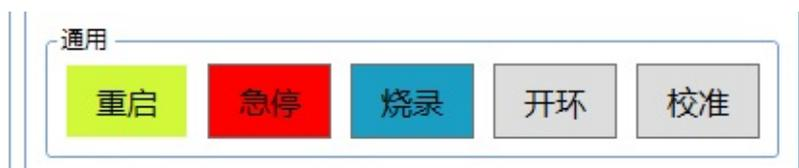
After opening the serial port, click "Flash" to set the drive to flash mode. After entering the flash mode, please close the drive software and continue to the next step.
