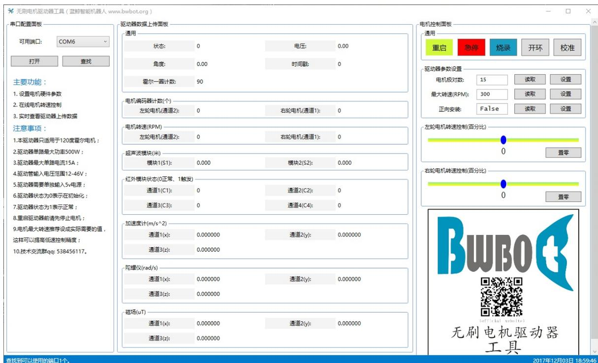
The software interface is mainly divided into three areas: serial port configuration panel, data preview panel, and control panel. The size of the interface can be adjusted arbitrarily. The blue status bar at the bottom of the interface will provide real-time feedback information according to the operation. Please pay attention to the actual prompt content.
