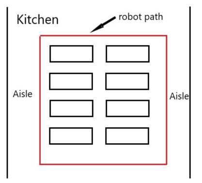
There are aisles on either side and tables in the middle. We can remotely control the robot to follow the red route first clockwise. Turn counterclockwise after the client prompts "Closed Loop Optimization Complete". Closed-loop optimization is also required. In this way, we can get a better map.
