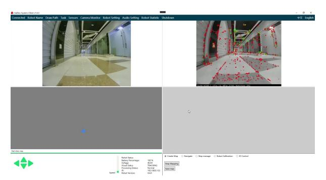
Now control your robot move around the target area. Please do not turn left/right without pressing front key or back key, it will make the visual system lost target.
