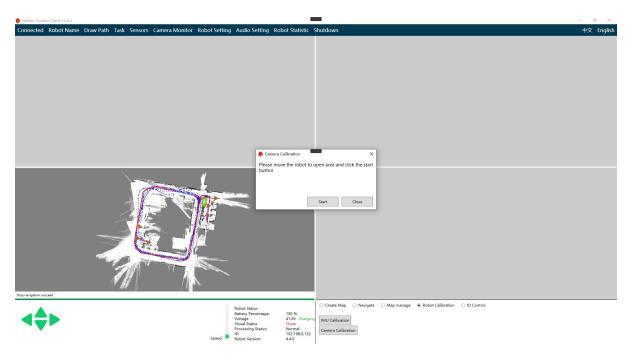
According to the prompt, remote control the robot to a more open position. Then click the start button.
