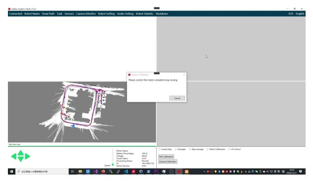
According to the window prompt, move your robot forms a closed-loop.
