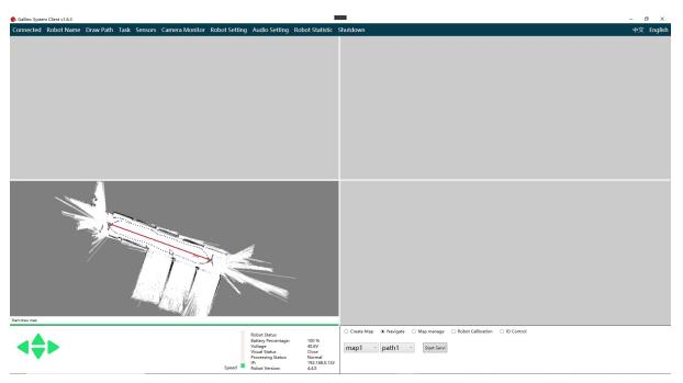
Control the robot move to the position that can be tracked, the robot must be on the navigation path, and the orientation of the robot must be consistent with the orientation of the mapping.
