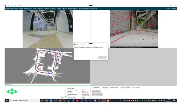
Wait for the closed-loop to complete, and then continue to move forward for a distance. At this time, the robot will automatically calculate the calibration parameters and errors.
