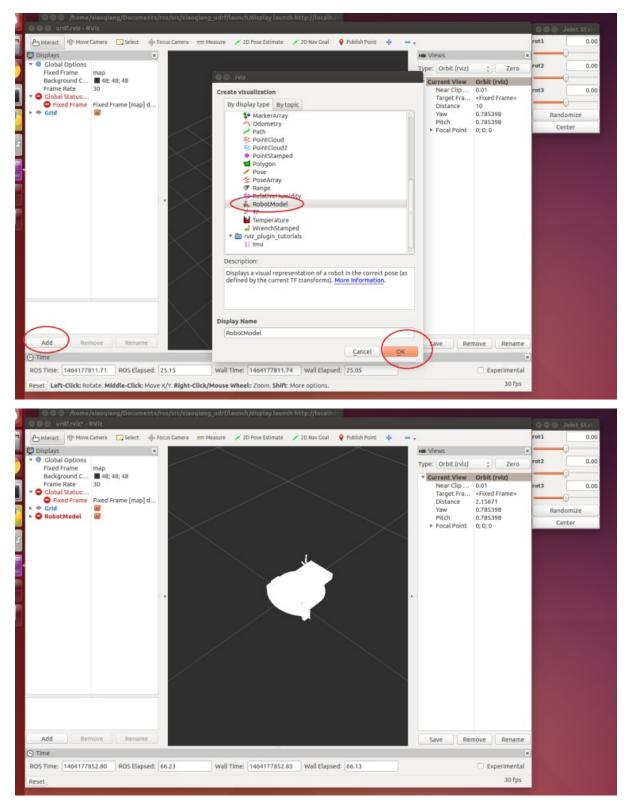
There is still a problem, the entire model is transparent and whitish, this is because the global coordinate system fixed frame in the rviz is not set properly, After map is changed to <code>base\_link</code>, it will display normally
