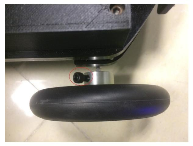
Solution: Re-tighten the screws in the figure above
