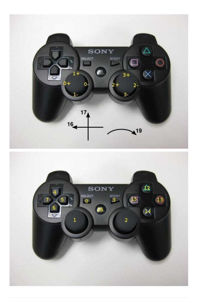
According to these button numbers, the relevant parameters in the launch file can be modified to change the button mapping relationship
