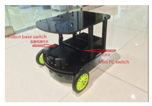
Place the battery flat on the free area in front of the host (the battery is blocked by two small black blocks).Connect the platform power cord according to the wire label. Installing computer host wifi antenna. USB camera and platform USB communication cable can be connected to the host's USB interface
