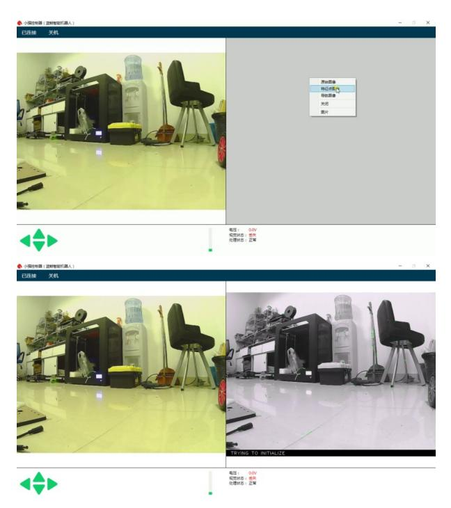
In the figure above, the left image is the camera's original color image, and the right side is the ORB\_SLAM2 processed black and white image. ORB\_SLAM2 has not been initialized successfully in the image, so the black and white image has no feature points. Hold down the "w" key to start the remote control Xiaoqiang, slowly move forward, so that ORB\_SLAM2 initialized successfully, that is, black and white images began to appear red and green features.
