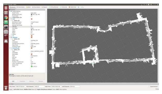
The idea of this article: Because it is a large-scale mapping, wifi network coverage is a problem, so we use the Bluetooth joystick to remotely control the robot movement. During the remote control, the lidar data was recorded through the rosbag. The joystick controlled robot ran a circle within the area and finally play the bag for map creation.
