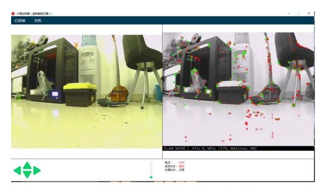
It is now possible to remote control of Xiaoqiang, and create a map of the surrounding environment. During the remote control process, it is necessary to ensure that the black-and-white image always has red and green feature points. If it does not exist, it means that the visual had lost, and it is necessary to remotely control Xiaoqiang to return to the place where the last missed lost position.
